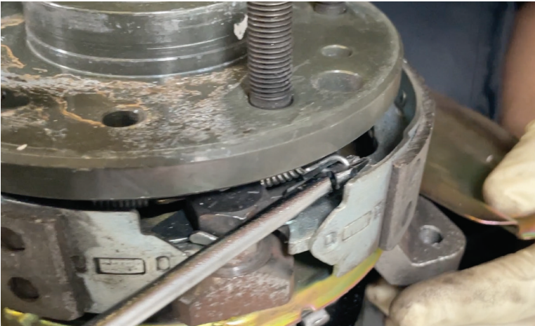
FIG. 1 - Remove upper spring first.
