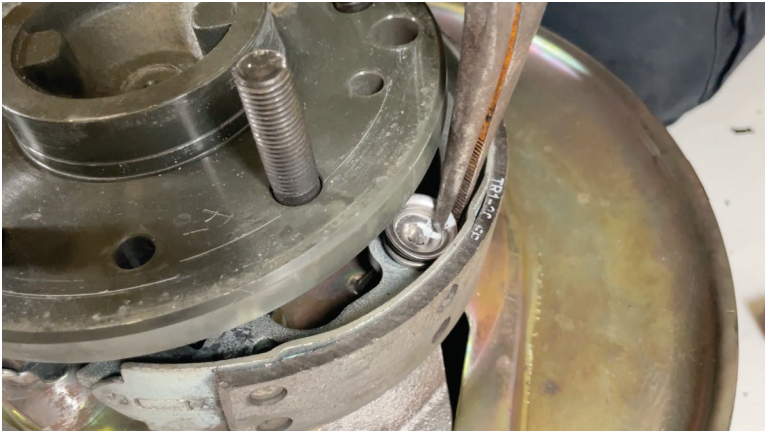
FIG. 3 - Install spring and spring cup on the shoe retaining spring
