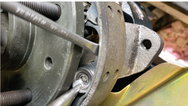
FIG. 2 - Remove spring cup by turning 90 degrees
