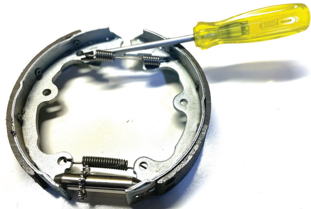
FIG. 4 - Build the parking brake assembly before installing. Above image shows how to install the upper spring after on the bearing assembly
