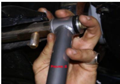
Moving toward the front side of the arm you can install the aluminum cradle bracket that is supplied w/2 7/16-20-1" Allen head bolts and lock washers. You are to re-use your existing 2 hole plate that come on the car. You will need a 3/8" Allen head socket/wrench/T-handle to tighten these down. (Figure 3) Do not torque these yet as you should move to the rear bolt again and torque it 1st. Torque the rear bolt to 60 ft/lbs. (oiled) and the front bolts to 40ft/lbs. (oiled) Oiled=Anti-seize
