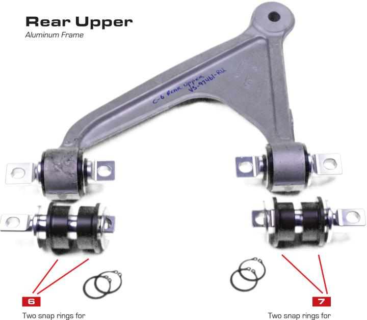
Two snap rings for the inner retainer
