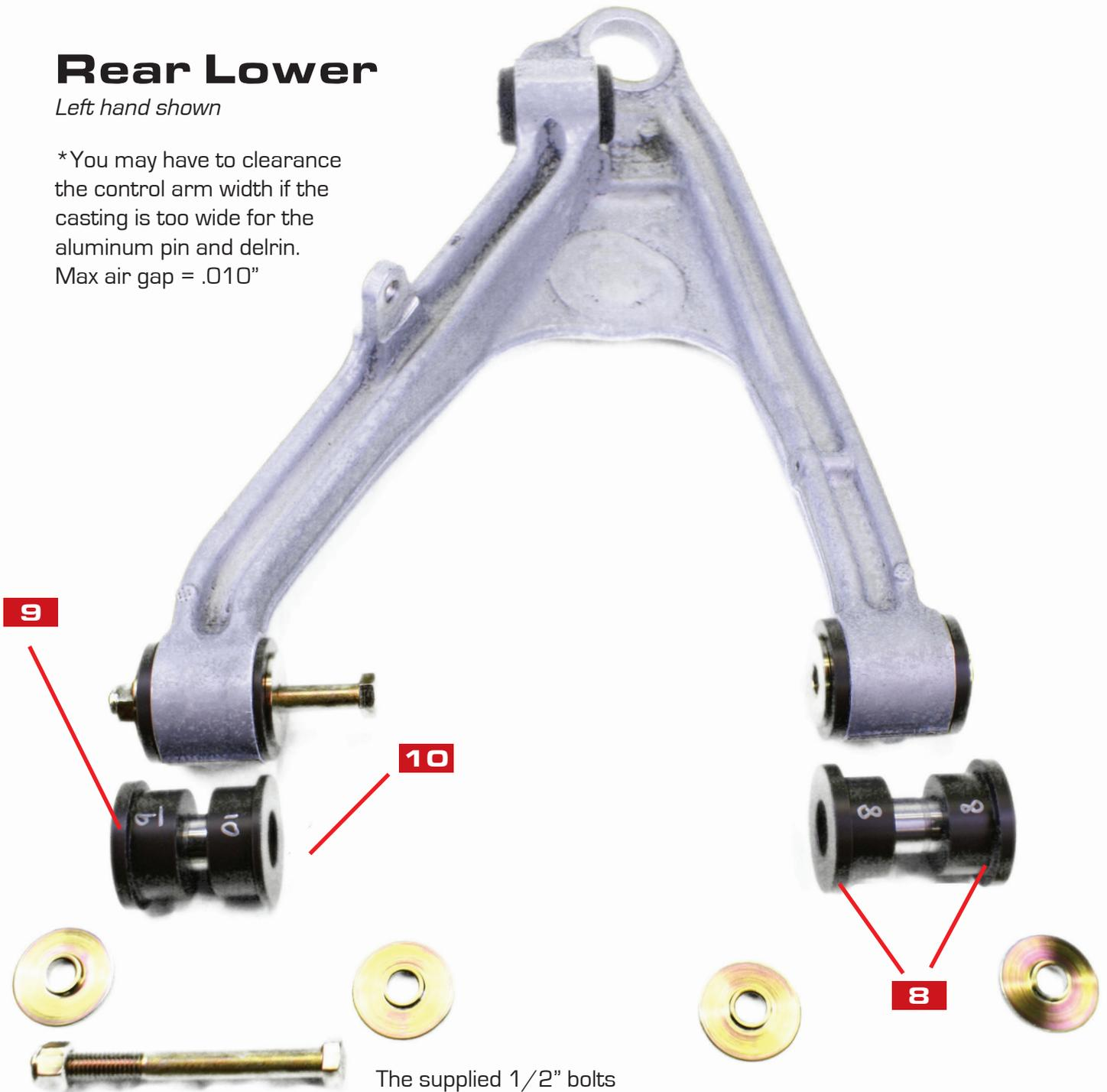
The supplied 1/2" bolts will pass through bushings marked #9 & 10.
