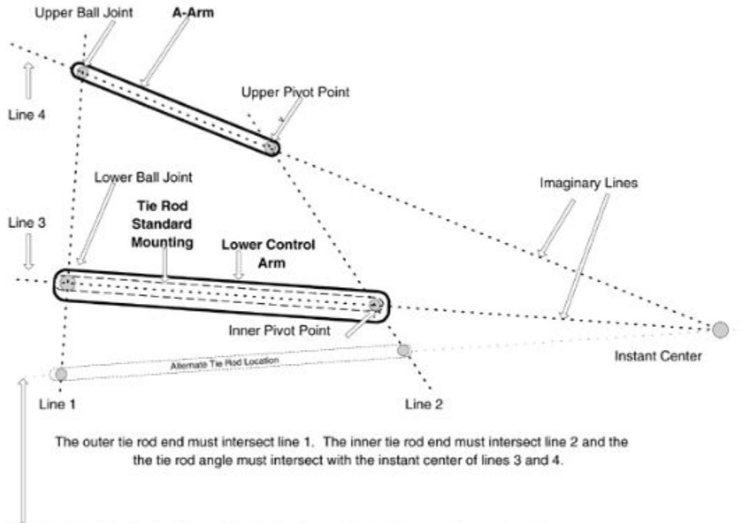
The tie rod could be located in an alternate location and still achieve zero bump steer. You could place the outer tie rod end anywhere on Line 1 as long as the inner tie rod landed on Line 2 and the tie rod angle intersected with the instant center.
