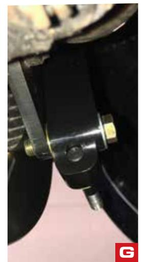
Once installed, you need to check the pad to rotor clearance ensuring both sides of rotor have equal distance from the pad to rotor all along the pad mating surface. Also check for clearance from the pads to the edge of the rotor. See **Photo D** for desired result. **Photos E & F** show installing the shims, **Photo G** is the bracket completed after final fitment and torqued to 70 ft lbs.
