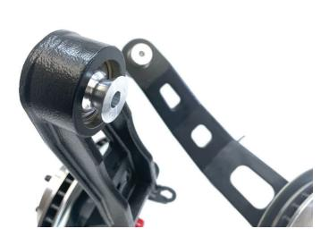
Remove your factory t-arm from your bearing assembly. You'll have to remove the parking brake harware and shoes to remove the four nuts on the t-arm studs.
