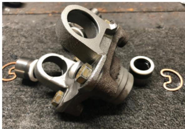
The Half Shaft flange can bend during install. You must secure the flange before pressing out and pressing in the u-joint. We recommend bolting it to your spindle flange.
