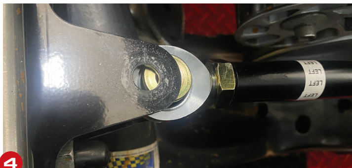
Rod end assembly should slip right into the bracket
