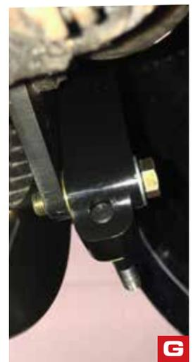
Once installed, you need to check the pad to rotor clearance ensuring both sides of rotor have equal distance from the pad to rotor all along the pad mating surface. Also check for clearance from the pads to the edge of the rotor. See **Photo D** for desired result. **Photos E & F** show installing the shims, **Photo G** is the bracket completed after final fitment and torqued to 70 ft lbs.
